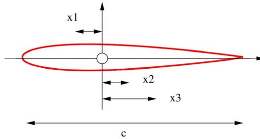
Figure 16 shows a sketch of the blade section, referred to the pitch axis;  $x_1$  is the distance of the aerodynamic center from the pitch axis;  $x_2$  is the distance of the elastic axis from the pitch axis;  $x_3$  is the distance of the center of mass from the pitch axis.
