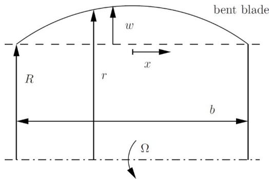
It is assumed that the blades are simply supported at both ends, as sketched in Fig. 17. Similar considerations apply to different arrangements.
