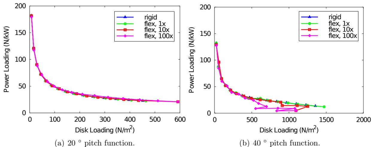
Figure 12. Comparison of rigid and flexible blades.
