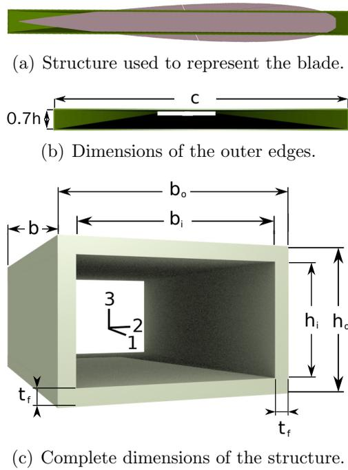
**Figure 7. Blade modeling as an extruded aluminum rectangle.**
