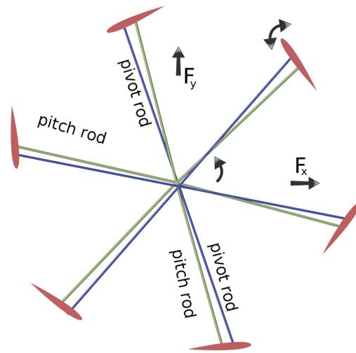
Figure 2. Sketch of cycloidal rotor working principle.
