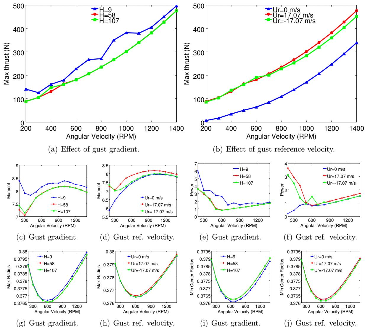
Figure 18. Effect of gust gradients and reference velocities.
