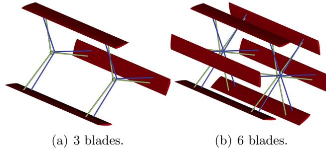
**Figure 9. Multibody models for different solidity configurations.**
